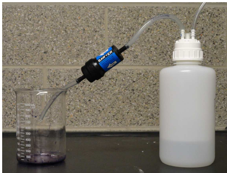
Figure 1. Pressurizing device for forcing challenge water through the Sawyer filter.
