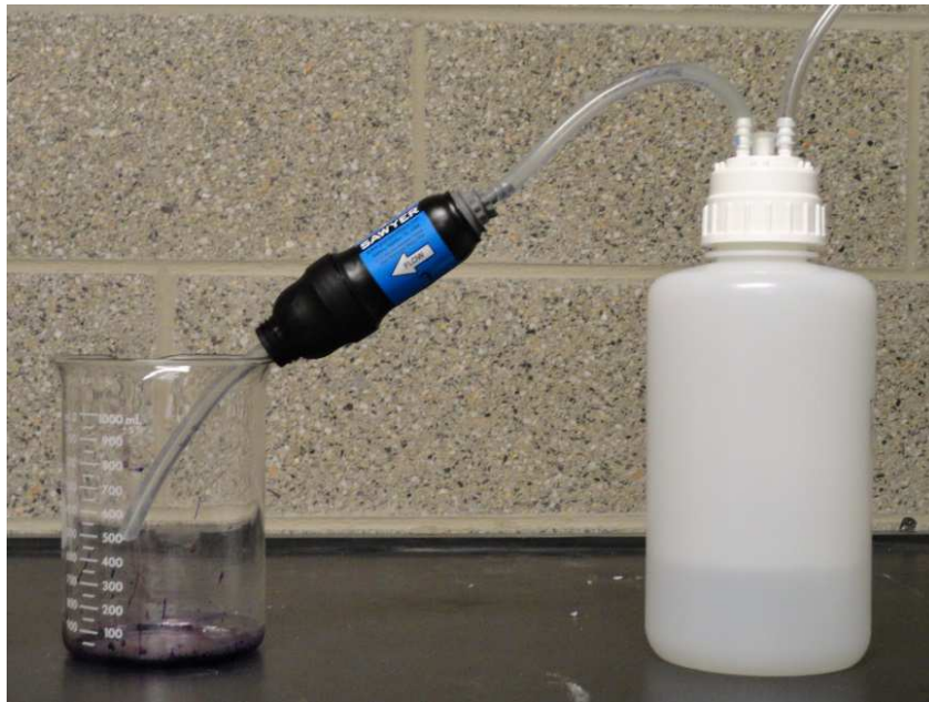
Figure 1. Pressurizing device for forcing challenge water through the Sawyer filter.
