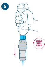
Squeeze forcefully and repeat as necessary until the filter is clean.
