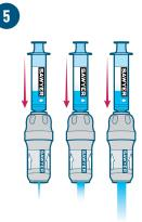
Forcefully backwash the filter a couple times with clean water.
